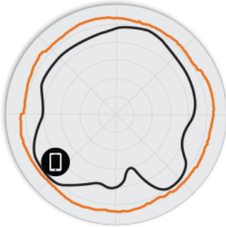
Figure 2. 2.4GHz Azimuth Antenna Patterns
