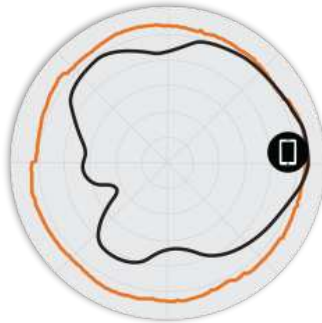
Figure 3. 5GHz Azimuth Antenna Patterns
