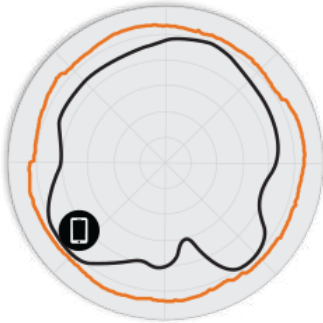
Figure 2. 2.4GHz Azimuth Antenna Patterns
