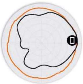
Figure 3 - T310d 5GHz Azimuth Antenna Patterns
