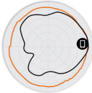
Figure 3. 5GHz Azimuth Antenna Patterns
