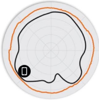
Figure 2. 2.4GHz Azimuth Antenna Patterns
