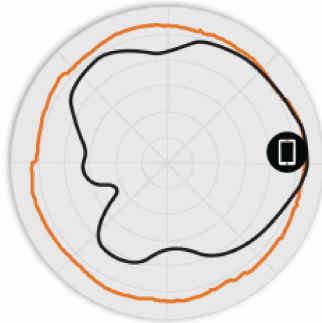
Figure 3. 5GHz Azimuth Antenna Patterns
