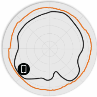
Figure 2. 2.4GHz Azimuth Antenna Patterns
