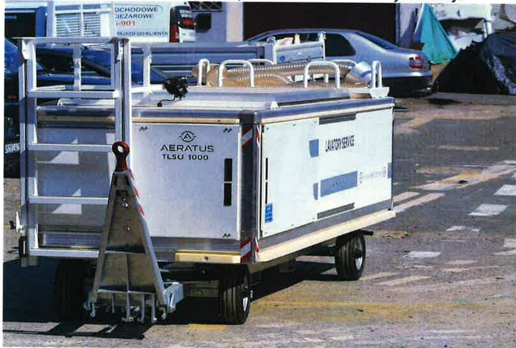
Fig.2 Front view with towing hook, ladder and lamp
