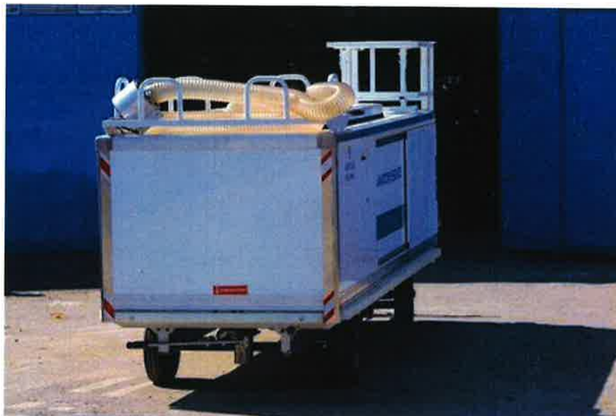
Fig.1 Rear view of the unit with lavatory hose and heated socket for aircraft connector
